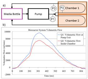
highly pulsatile with specific waveforms. Moreover, our recent findings suggest that fluid oscillations induced from pulsatile flow are important in enhancing valvular matrix generation and gene expression [3]. Our current updates to the bioreactor system will permit physiological components of pulsatile flow-induced oscillations to be used for conditioning developing, 3-dimensional engineered valve tissue constructs.
