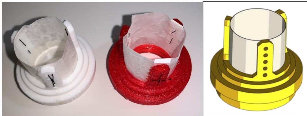
Figure 25. 3D printed valve holders in aortic tri-leaflet configuration with three posts
