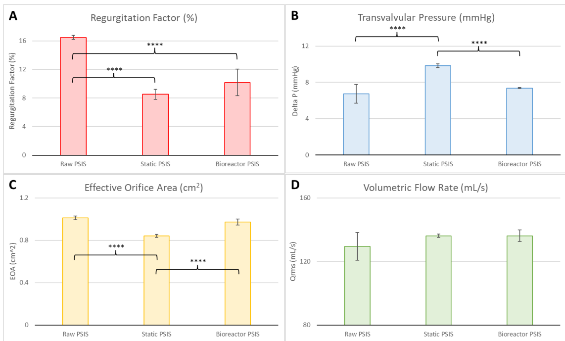
Figure 38. Hydrodynamic results of Raw PSIS valve, Static PSIS valve, and Bioreactor PSIS valve. (A) Regurgitation factor, (B) Transvalvular pressure, \Delta P , (C) Effective orifice area, EOA, and (D) Volumetric flowrate, Q_{rms} .
