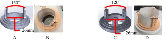
Cylindrical valves sutured onto customized valve holders (Mitral: A & B, Aortic: C & D), which are 3D printed with thermoplastic polyurethane (TPU) material.
